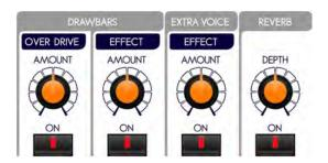
The <u>Effects</u> <u>Controls</u> are located in the upper right portion of the Control Panel, and consist of four Touch Tabs and a Rotary Control associated with each Touch Tab.
